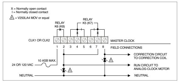
*Figure B-1 Three-Wire Synchronous (59th Minute, Dukane 24SS)*
